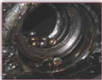
Catastrophic engine failure caused by IMS bearing failure
