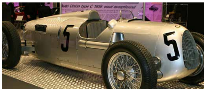
The Auto Union Type C, an audacious engineering feat, a V16 supercharged engine, which by 1936 grew to 6-liters, producing 520 bhp, allowing speeds of well over 200 MPH.
